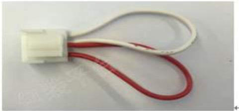
Fig.2 short wiring (new)
